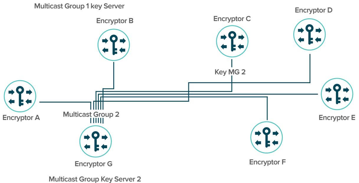
Each multicast group has its own key and up to 256 individual multicast groups are supported. Broadcast frames are treated as a “special case” of multicast and are all encrypted using the same broadcast key.
