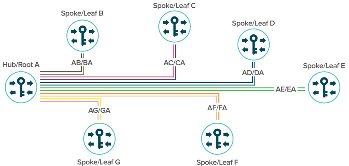
Senetas key management supports the combination of a pairwise key system with a group key system, so multicast frames can be encrypted with a group key when using a point-to-multipoint topology. For unicast frame encryption, pairwise keys are used; while multicast frames are encrypted using the group key system.
