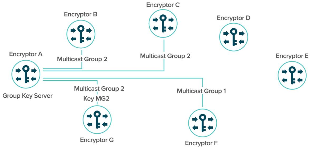
Each multicast group has its own key and up to 256 individual multicast groups are supported. Broadcast frames are treated as a “special case” of multicast and are all encrypted using the same broadcast key.
