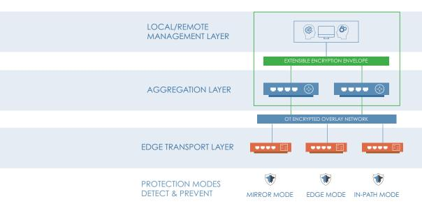
Project Orthos provides dual encryption security. First, a secure link from the management layer (wherever it is located) to the remote asset. Second, an encrypted overlay to the operational technology network infrastructure.
